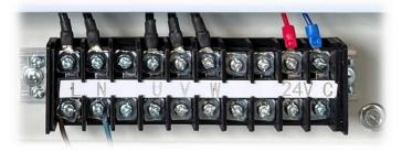
To access the terminals inside the DRIVE, (4kW and up) remove the lower front cover.
