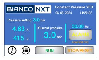
When the float switch falls to its OFF position, after the Pressure Setting - Parameter #17, Water Shortage Delay Time has elapsed a message will appear on the screen "Low Float Prot".
